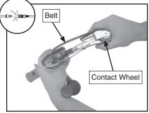
Figure 5. Preparing the sanding belt.
